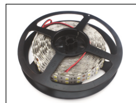
LED Strip: 3528LED, 240LEDs/M, 19.2W/M, double rows
